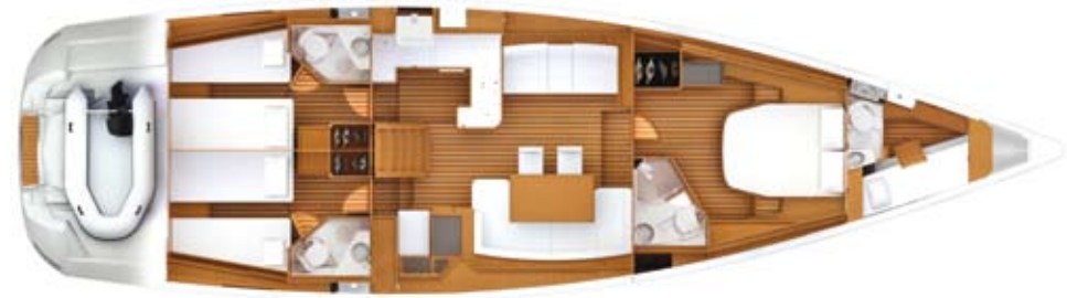
4 cabin version : 2 transformable cabins forward and 2 aft cabins. Optional forward cabin
